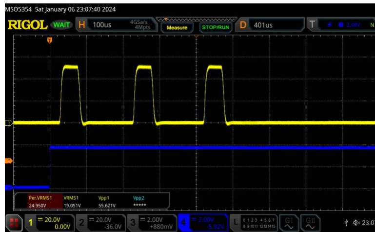
Simple pulse sequence using one pulse generator. Blue trace is trigger, yellow is DC bias CH1.
