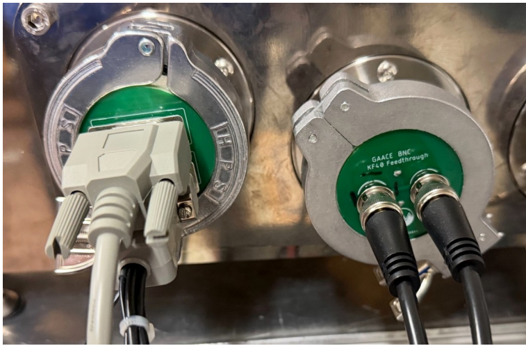
D9 and BNC KF40 feedthroughs installed on a vacuum chamber flange
