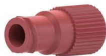
IDEX Threaded Luer Adapter, Red PEEK, 0.050 (in) Bore, Female Luer x Female 1/4-28 Flat Bottom
